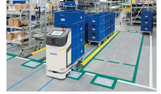
Fig. 5: The ActiveShuttle AMR by Bosch Rexroth. The top-view robot shape is outer-approximated by a circle.
